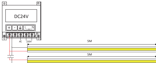
Monochrome temperature wiring diagram 1: Power + lamp belt connection mode
